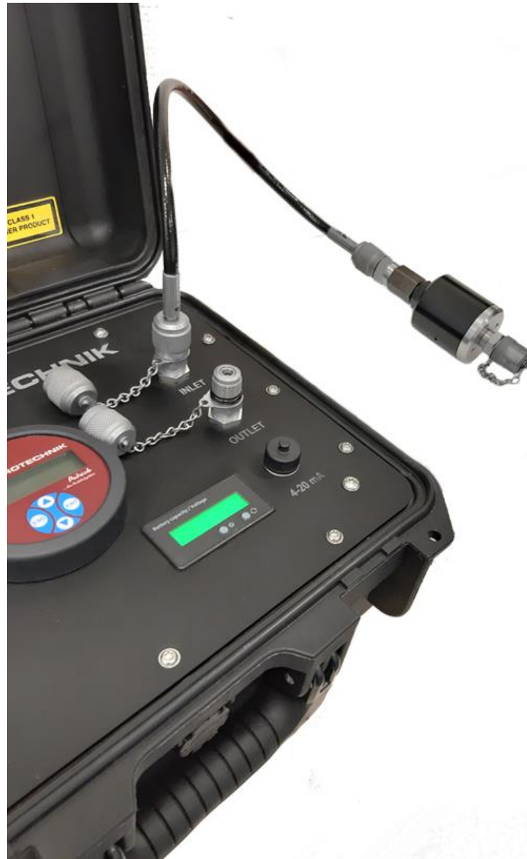
Figure 7: Connection to the pressure line via the pressure reducing valve
